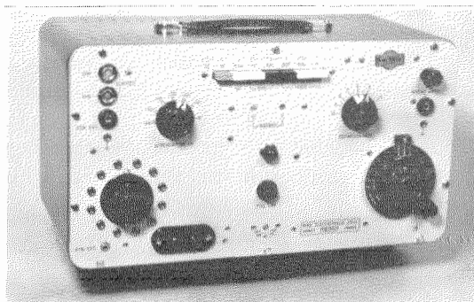
Figure 24—Test set for 625- and 819-line European television receivers.
